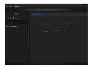
When connection succeeds, AGS-i Touch downloads configuration information from control box. Navigate back to the main screen, you can see any groups that have been configured along with all encoders listed at the bottom.
