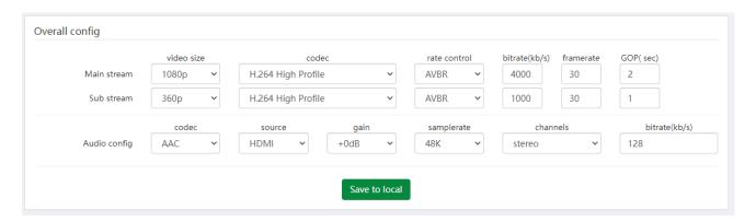
The basic parameters of video coding are shown here, which are used to quickly and uniformly modify the system settings of all devices. After configuring the system settings, click the "Apply this unit" button to automatically set all the parameters of all devices to be consistent.
