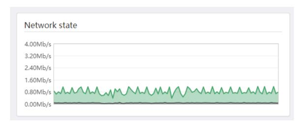
The network status shows the upstream and downstream status of the network card at that time. The dark green represents the upload rate (output stream), and the light green represents the download rate (input stream).
