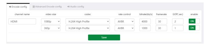
This is the same as some of the parameters of "All Settings", but each one corresponds to one encoding device. Each device can be set to different encoding parameters. The first line of each device parameter is the main encoding parameter, and the second line is the backup encoding parameter.
