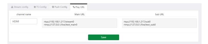
As shown in the figure above, here will organize all the playable protocol addresses in this interface according to the output protocol you currently open, so that it is convenient to copy to other playback systems for use.
