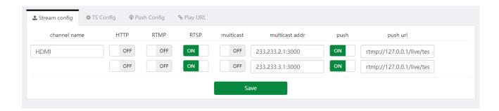
It is used to set the common output protocol switch and address of each channel, and the livestream broadcast address supports livestream streaming protocols such as rtmp/rtsp.
