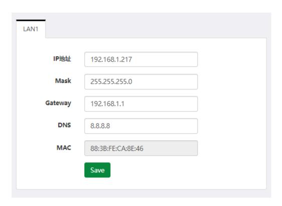
In the network settings, the original default IP address is 192.168.1.217, and the user can customize the fixed IP location. After applying, the newly set IP location must be used when connecting to the web next time.
