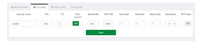
It is used to set the parameters of mpegts encapsulation in HTTP and multicast (UDP) protocols. For details, please refer to the definition of mpegts format.
