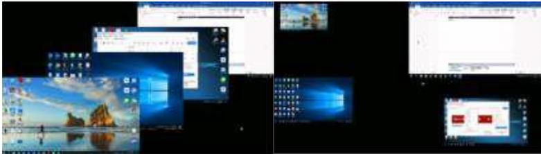
A free style of display includes picture-on-picture (PoP) up to 4 computers in separate windows on the monitor as default layout. Using the console mouse to resize and re-position each window on the screen and can be saved.
