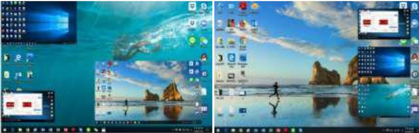
A quad PiP view has up to 4 computers on the monitor with one computer as the main display and the other three which can be resized and re-positioned by using the console mouse overlapping the main display in inset windows.
