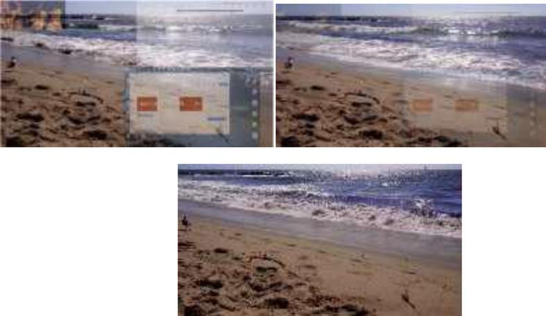
At PiP display, one computer as the main display and others as sub-display can be transparent by mouse wheel roll down or up. The transparent function only apply in one full display with other sub-display (pip) mode.
